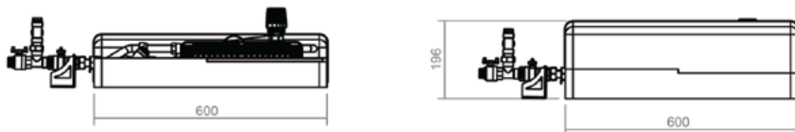
Figure 3. The dimensions of the HIU-DHW
